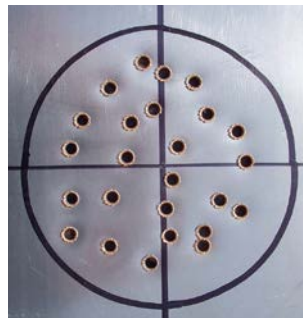
Testing MIL-SAMIT Part 1 - .30 cal 7.62 NATO M80 25 shots in an 8-inch circle
